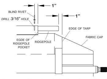
**STEP 4:** Install rivet 1" from edge of pocket. Pull tarp to full length and install second rivet 1" from opposite end of pole.
