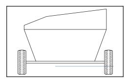
NOTE: If ordering galvanized caps, make sure the box is flat across the top. The above illustration shows a box with an uneven angle across the top. Galvanized caps will not fit this box; you must order fabric caps.
