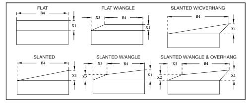
NOTE: Flat caps can only be used on a SLANTED extension (see above), and the side walls must be vertical.
