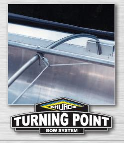
Easy Release and Capture Spring loaded locking pins make locking and unlocking the bows as easy as pulling a rope. Pull the rope to release the pin allowing you to pull the bows to the side in the open position. When done loading simply pull the bows across the load and let the locking pins capture the bows and lock them into position.
