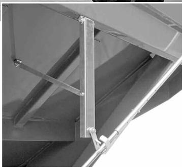
*Above and closeup at left: The Universal Retainer Support Kit lets you position the crank arm in the most efficient spot.*
