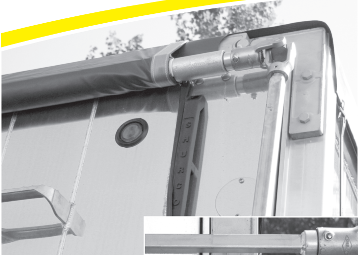
Above: The Wil-Slip™ Joint hooks into place flat against the trailer.
