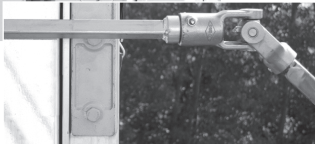
Above: The Wil-Slip™ Joint hooks into place flat against the trailer.
