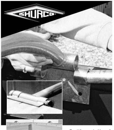
Top: When used with a rollaway ridgepole, Heavy-Duty Bows can be spaced up to 12 feet apart for more wideopen loading.
