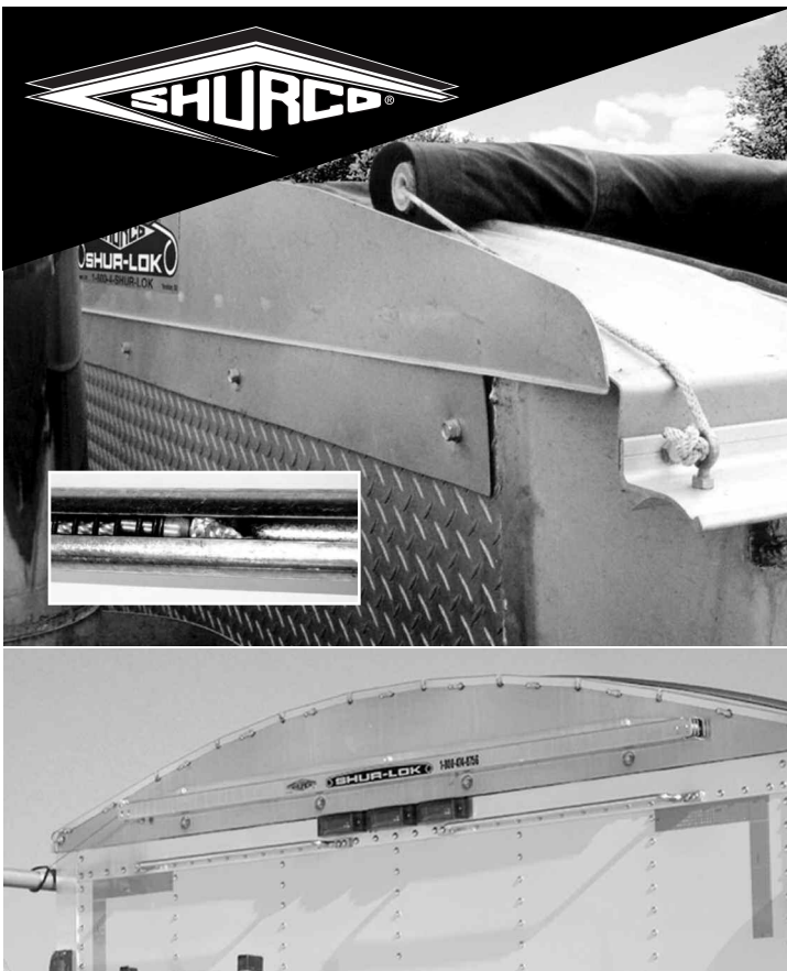
Top: The Shur-Return™ features a heavy-duty steel tension spring (inset).
