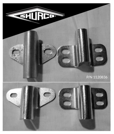
Top: The old bow bracket design is pictured on the left. The new bracket's top hole is used on box rails that are 3 inches or less while, for box rails that are over 3 inches in width, the bottom hole is used.
