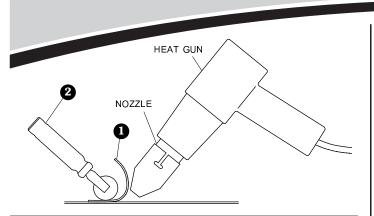
Verify **Shur-Pro® Tarp Repair Kit (P/N 1108059)** includes heat gun, nozzle and scissors, along with part numbered items listed below.
