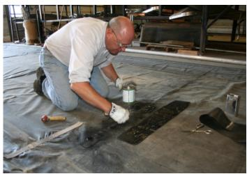
STEP 5: Press patch on tarp, then allow glue to set for 1 to 24 hours.
