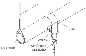
STEP 5: U-Clamps: Position tarp flush with front end of roll tube. Square up tarp along roll tube to match length of tarp on fixed tube. Mark U-clamp locations 6" from each side of web/cable assemblies. Install U-clamps with 1/4" x 3/4" self-drilling screws.
