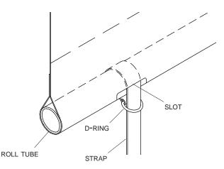
**STEP 5:** U-Clamps: Position tarp flush with front end of roll tube. Square up tarp along roll tube to match length of tarp on fixed tube. Mark U-clamp locations 6" from each side of straps. Install U-clamps with 1/4" x 3/4" self-drilling screws.
