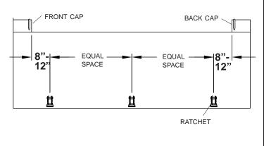
**STEP 2:** Mark and drill 5/16" holes. Fasten with 3/8" x 1" self-tapping screws, lock washers and nuts.
