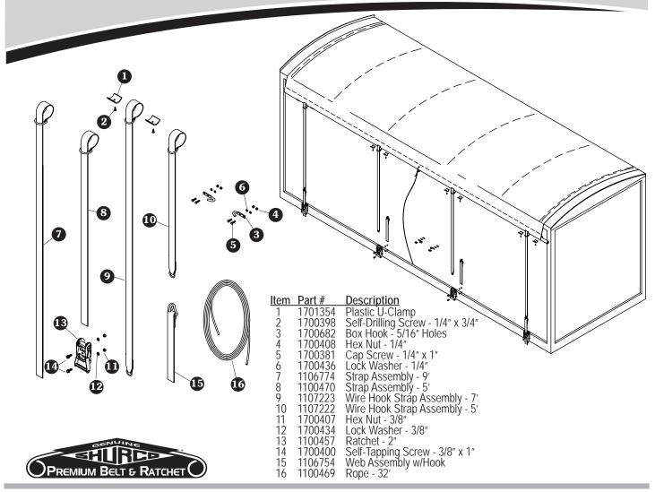
STEP 1: Ratchets: Position ratchet 8" to 12" from front cap at convenient operating height. Locate second ratchet 8" to 12" from back cap at same height. Equally space remaining ratchets.
