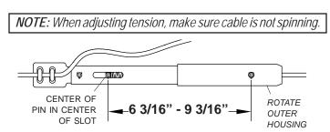
**NOTE:** If this dimension is under 6 5/8" on initial stretch, consider restretching cable to allow for more adjustment as cable stretches.
