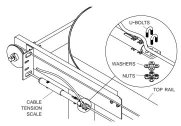
**NOTE:** Cable tension scales must face same direction on both driver and passenger side. Cable tension scale must be placed on lower cable.
