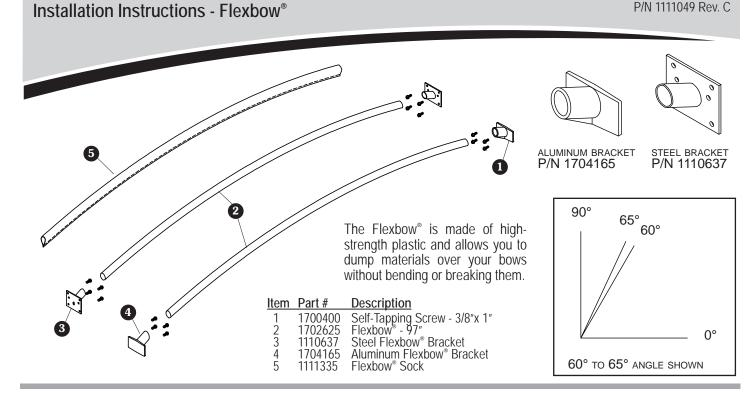
**STEP 1:** Equally space bow brackets on each side of trailer. Mount brackets flush with top rail. Pre-drill 5/16" holes and secure each bracket with four (4) self-tapping screws.
