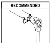
**NOTE:** U-joint is designed to operate as shown at right and is considerably stronger in this position.
