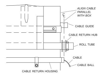
**NOTE:** Cable coming off cable return hub must align with center of cable guide so cable runs parallel to truck.
