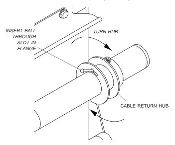
STEP 12: Mark cable with tape at top of cable return housing where cable exits. Turn cable return hub, wrapping four more inches of cable around hub, to add tension to cable. Tighten both set screws.
