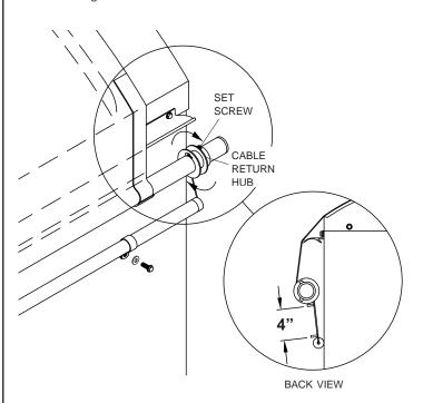
**STEP 13**: Adjust alignment of cable return hub and cable guide, if necessary. Loosen set screws on cable return hub and adjust position of hub, while keeping cable under tension.
