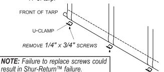
STEP 4: Insert Shur-Return™ into roll tube at front of trailer, with rope at open end of roll tube. Thread rope through nylon end plug. Reinstall U-clamps with 1/4" x 1/2" screws.
