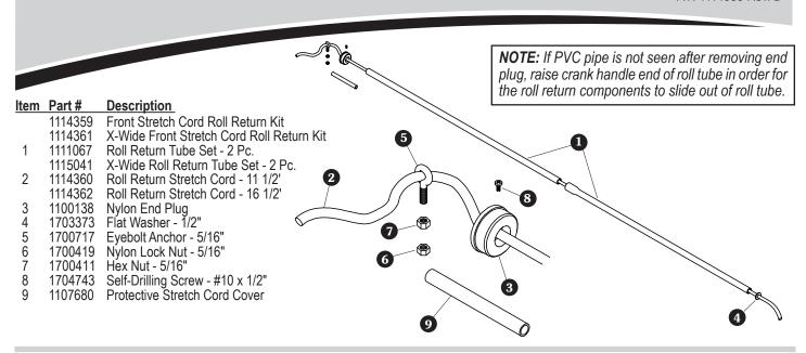
**STEP 1:** Press belled PVC pipe over end of straight PVC pipe. Press end plug into end of straight pipe.
