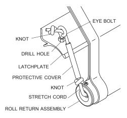
**STEP 9:** Test operation. Cut excess stretch cord and melt any frayed ends.
