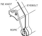
STEP 7: Insert Shur-Return™ rope through eyebolt, remove all slack from rope and tie knot. Cut
