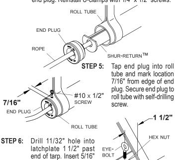
STEP 6: Drill 11/32" hole into latchplate 1 1/2" past end of tarp. Insert 5/16" eyebolt through hole and secure with hex nut and nylon lock nut.
