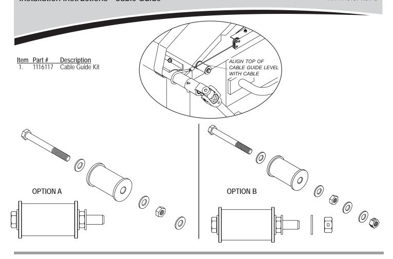
STEP 1: Assemble parts onto 3/8" x 3 1/2" cap screw as shown.
