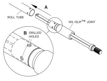
B. Weld into drilled holes, filling holes with weld until flush with roll tube.
