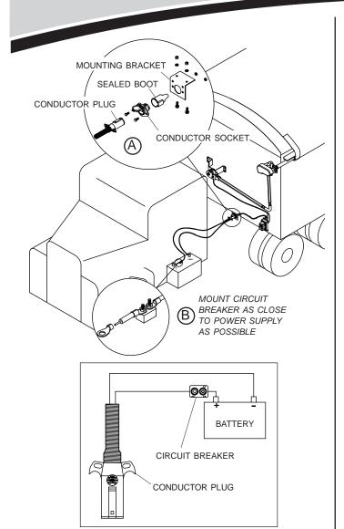
**STEP 1: Conductor plug.** Unfasten and remove insert from conductor plug. Feed 6-ga. wire through plug and into brass contacts on insert. Tighten set screws to secure wires. Replace insert into conductor plug and secure screw.
