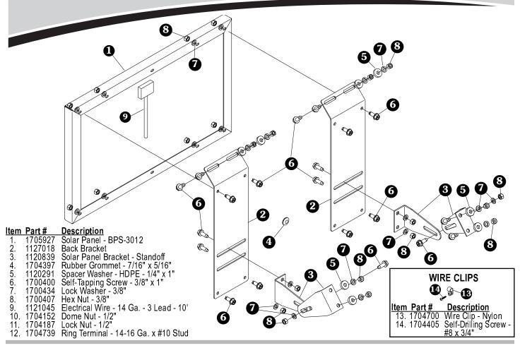
STEP 1: Determine solar panel location on trailer. Locate panel toward passenger side of trailer. Hold panel and back brackets against trailer, aligning slots in back brackets with horizontal and vertical rivet lines on trailer. Mark rivets that need to be removed. If slots cannot be aligned with rivets, drill 5/16" holes for fasteners.
