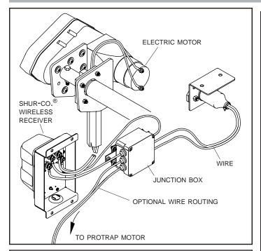
USE DIELECTRIC GREASE (PART #1704378) TO PREVENT CORROSION ON TERMINALS.
