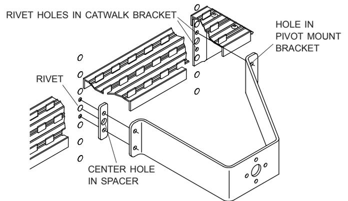
**STEP 3:** **Fasten -** Realign pivot mount bracket and spacer with holes in catwalk bracket and trailer. Fasten with 3/8" x 1 1/2" cap screws, flat washers, lock washers and hex nuts.
