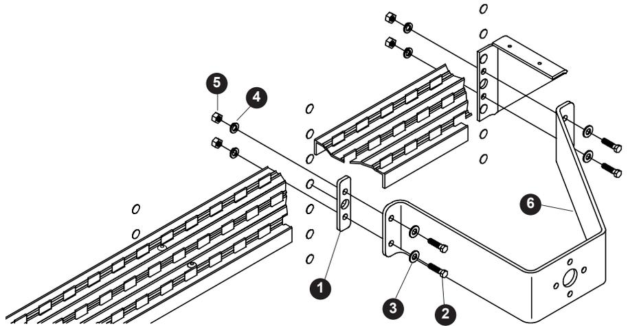
**STEP 1:** Remove two rivets from bracket on driver's side of catwalk. Rivet holes will be used to fasten pivot mount bracket to trailer.
