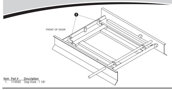
STEP 1: Weld stop hooks 1" from rack. Edge of hook should contact existing plastic wear plate.
