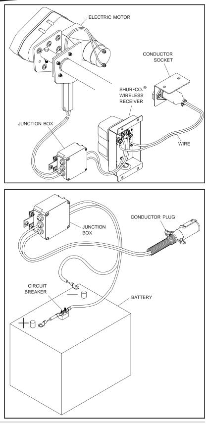
Cab: Remove solenoid, rocker switch, and 14 ga. wire. Install junction box between battery and conductor plug.
