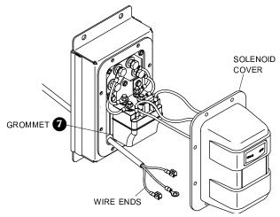
**STEP 6:** Remove washers and nut from negative post on solenoid and place ring terminal **4** over post. Re-fasten washers and nut over ring terminal on negative post.
