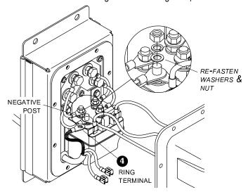
STEP 7: Remove female quick disconnect **3** from left male spade connector on solenoid. Press piggyback quick disconnect **3** onto left male spade on solenoid.
