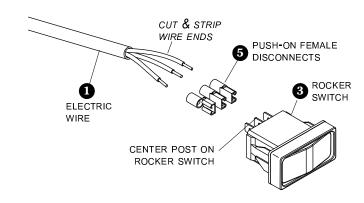
STEP 4: On opposite end of electric wire ①, crimp ring terminal ② to wire, connected to center post on rocker switch ③. Crimp piggyback quick disconnects ③ to remaining two wire ends.
