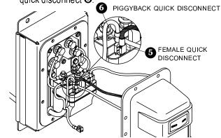
**STEP 9:** Repeat steps 7 and 8 on male spade connector on right side of solenoid. Re-connect power to battery.
