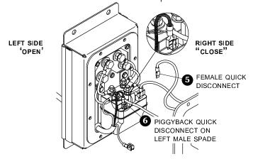
**NOTE**: Left male spade connector on solenoid connects to "Open" side of rocker switch on solenoid cover. Right male spade connector connects to "Close" side of switch.
