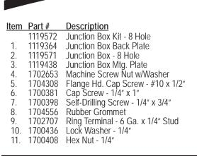
Routing wires through the sealed junction box greatly reduces corrosion on wire connections. Used with the 3500 Series and ProTrap® systems.
