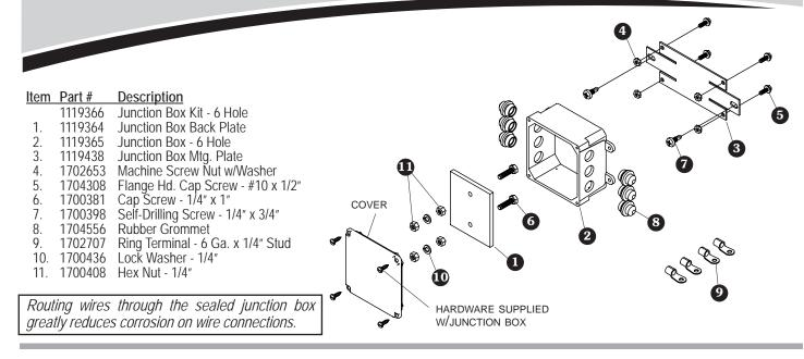
STEP 1: Insert 1/4" X 1" cap screw through holes in back plate and secure with nuts.
