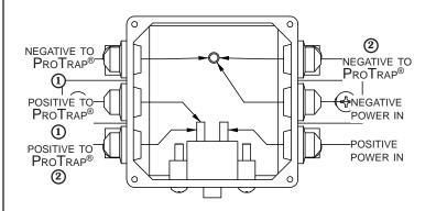
**STEP 9:** Fasten cover to junction box with supplied screws.
