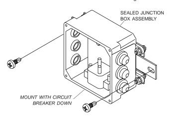
**STEP 7:** Pierce grommets with ballpoint pen so that terminal wires can be inserted through pierced holes.
