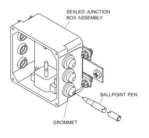
**STEP 8:** Run 6 ga. wire from conductor socket to junction box. Crimp 1/4" ring terminals to wire ends. Remove hex nut and lock washer from junction post assembly. Place positive wires on positive post and negative wires on negative post. Secure with hex nuts and lock washers.
