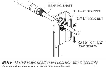
fastened to roll tube extension as shown.
