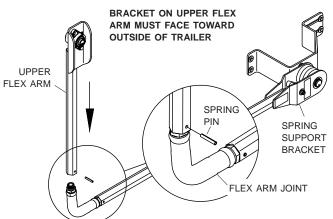
**STEP 9:** Slide bearing shaft on Gate Flex<sup>™</sup> through flange bearings on upper flex arm. Refasten 5/16" x 1 1/2" cap screw through hole in Gate Flex<sup>™</sup> and secure with lock nut.
