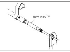
PO BOX 713 = 2309 SHUR-LOK STREET YANKTON, SOUTH DAKOTA 57078-0713 PH. 1-800-474-8756 = FAX 605-665-0501 **STEP 2:** At rear of trailer, remove 5/16" x 1 1/2" cap screw and lock nut from Gate Flex<sup>™</sup> bearing shaft. Loosen set screws in bearing, then carefully remove flex arm from bearing shaft.
