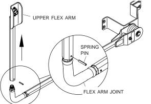
**STEP 4:** Unfasten and remove existing bearing flush mount from bearing mount plate on upper flex arm.
