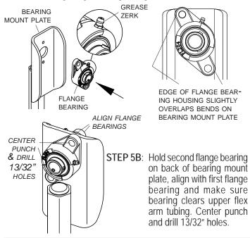
PO BOX 713 = 2309 SHUR-LOK STREET YANKTON, SOUTH DAKOTA 57078-0713 PH. 1-800-474-8756 = FAX 605-665-0501 **STEP 7:** Fasten flange bearings to bearing mount plate with 3/8" x 2" cap screws and lock nuts.
