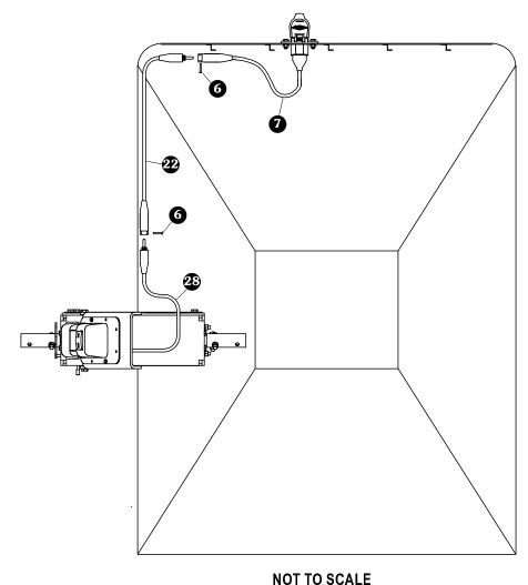
**NOTE:** Coat each connection with dielectric grease (P/N 1704378) to prevent corrosion.
