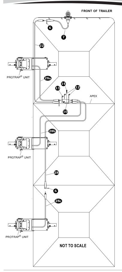
**NOTE**: Coat each connection with dielectric grease (P/N 1704378) to prevent corrosion.
