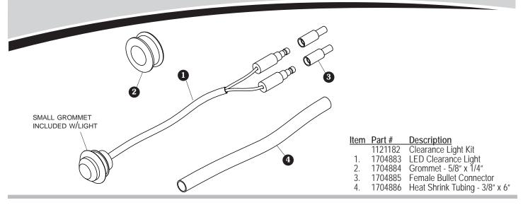
STEP 1: Disconnect power to trailer. Unfasten clearance light from front of trailer.
