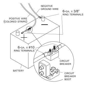
**STEP 6:** Crimp 3/8" ring terminals to positive and negative wires as shown and connect wires to battery.
