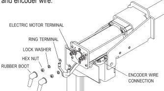
**STEP 3:** Unfasten and remove only 5/16 inch lock washers and hex nuts holding motor to motor bracket/front arm assembly, leaving motor mount bearing retainers in place.
