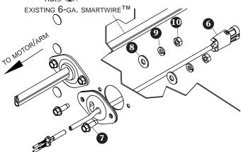
STEP E: Fasten weather pack connector **●** to end of encoder wire **⊙**, connecting side **A** to white wire and side **B** to black wire.
