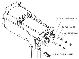
STEP L: Plug encoder wire **6** into encoder wire on motor. Secure with cable tie **9** to prevent wire damage.
