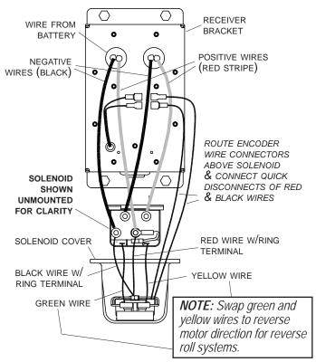
STEP 8: Reconnect power to receiver. Pair (introduce) SMART2<sup>™</sup> remote to receiver as shown in remote instructions (P/N 1122198) and verify operation.
