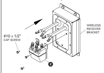
STEP 4: Remove receiver bracket from trailer and install encoder wire 12 through drilled hole from back side of bracket. Feed one connector at a time through drilled hole.
