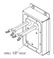
STEP 3: Install solenoid **②** onto wireless receiver bracket. Fasten with #10 x 1/2" cap screws.
