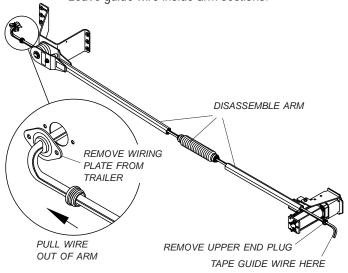
STEP F: Remove lower end plug and wiring plate from existing 6-ga. SMARTwire™. Discard wiring plate. Route blunt end of 6-ga. wire through wiring plate in new encoder wire assembly ③. Fasten wiring plate ④ to existing holes in front of trailer with screws ④, flat washers ④, lock washers ④ and nuts ④.
