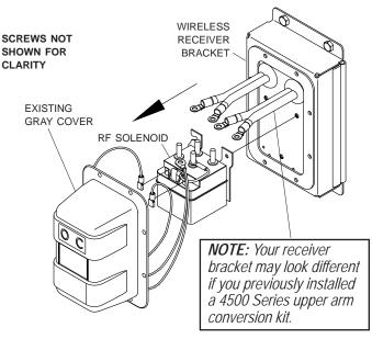
STEP 2: Using pilot hole in receiver bracket as guide, drill 1/2" hole in bracket.
