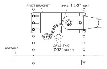
STEP C: Align new wiring plate of encoder wire assembly **6** with 1 1/2" hole. Using wiring plate as guide, mark and drill two 7/32" holes as shown.
