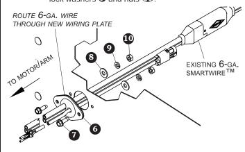
STEP G: Use drill or snips to enlarge hole in end plugs **3** so encoder wire will fit through hole along with 6-ga. wire. Run 6-ga. wire and encoder wire through hole.
