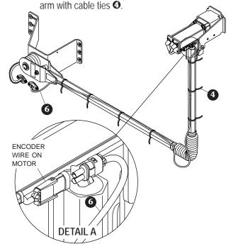
**STEP G:** Plug encoder wire **6** into encoder wire on motor. See detail A. Reinstall motor cover. Go to step 5.
