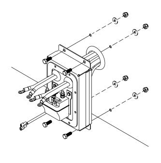
STEP 7: Connect wires from receiver bracket to solenoid and from gray solenoid cover to solenoid as shown below.
