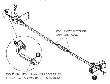
Fasten weather pack connector **●** to end on encoder wire **⑤**, connecting side **A** to white wire and side **B** to black wire.
