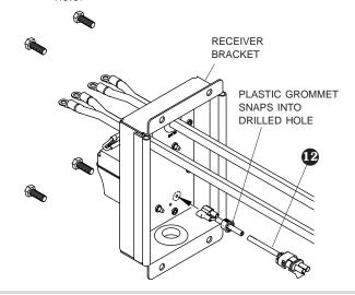
Install encoder wire up arm to motor.
