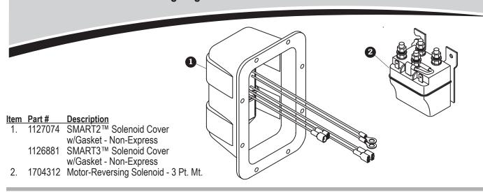
**STEP 1:** Disconnect power to receiver. Remove existing gray cover and RF solenoid from receiver bracket.
