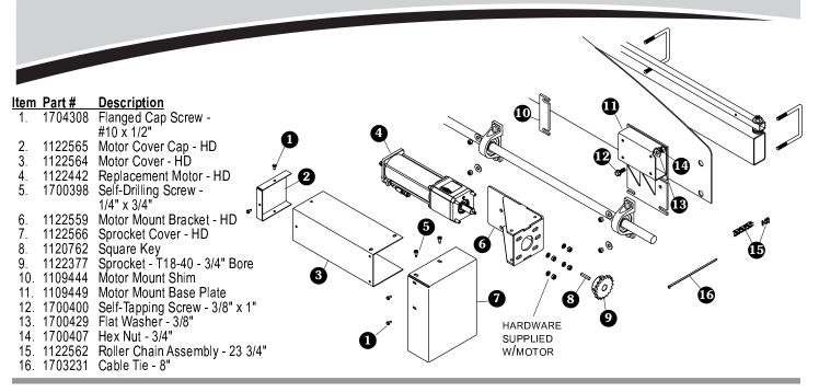
STEP 1: Loosen driver side bearing on front drive assembly. Slide base plate behind bearing. Square up mount and retighten bearing.
