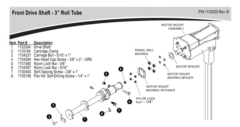
STEP 1: Loosely fasten cartridge clamp ② to drive shaft ● with screw ❸ and lock nut ④. Insert drive shaft into roll tube as shown. To secure drive shaft to roll tube, tighten nut ④ to 20 ft\*lbs.
