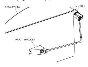
**STEP 6:** Align flex arm vertically with front of trailer and 90° to roll tube.
