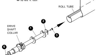
STEP 2: Install three screws ③ through roll tube and flats on drive shaft collar. Drill 5/16" hole between flats and collar, then fasten screw ④ through roll tube and drive shaft collar.
