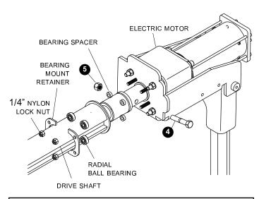
**NOTE:** Make sure all fasteners holding motor to upper flex arm bracket are tightened securely.
