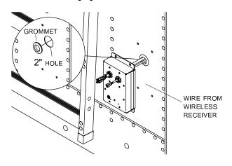
STEP 10: Align holes on wireless receiver with holes on trailer. Fasten receiver to trailer with 5/16" x 7/8" cap screws, lock washers and nuts.
