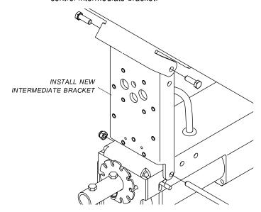
**STEP 5:** Install rubber grommets into intermediate bracket.
