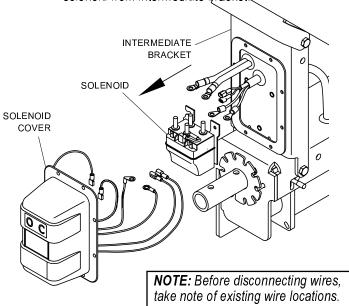
STEP 3: Remove wires and grommets from existing intermediate bracket. Unfasten and remove intermediate bracket from Protrap® unit and trailer.
