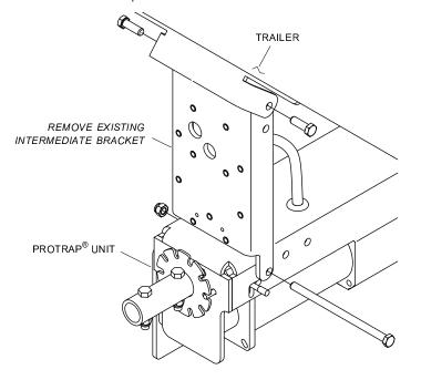
STEP 4: Replace existing intermediate bracket with new external control intermediate bracket.
