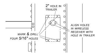
STEP 9: Install grommet into 2" hole. Insert wire from wireless receiver through grommet.
