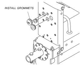
STEP 6: Insert wires through grommets. Install solenoid on bracket.
