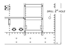
STEP 8: Align holes in wireless receiver over 2" hole in trailer as shown below. Using holes on flanges on receiver as a guide, mark and drill four 5/16" holes as shown.
