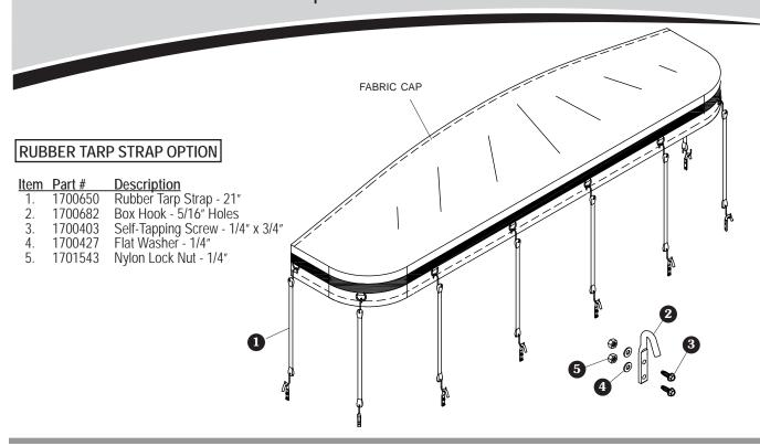
STEP 1: Apply small amount of lubricant to front groove on combo bow. Slide rod in fabric cap entirely into groove.
