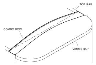
STEP 2: Center combo bow on trailer. Mark both sides of bow as shown, with no part of bow extending past side of trailer. Remove excess material from combo bow.
