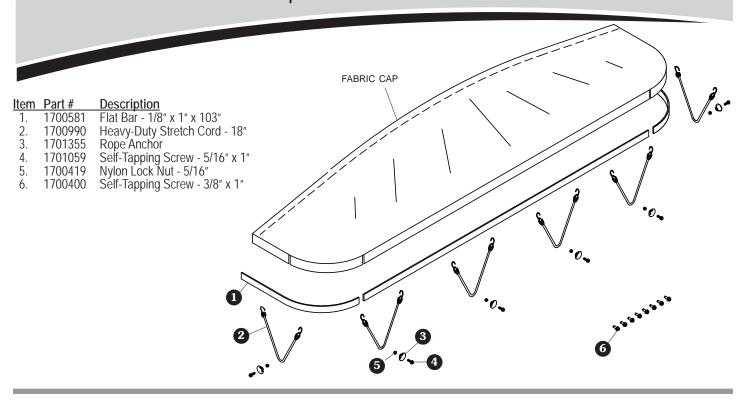
STEP 1: Apply small amount of lubricant to front groove on combo bow. Slide rod in fabric portion of cap entirely into groove.
