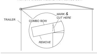
STEP 3: Center bow brackets under combo bow, against inside of trailer. Mark bracket locations and remove bow.
