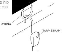
STEP 4: Locate box hooks so tarp straps receive at least 10 pounds of pressure. Drill 1/4" holes and fasten box hooks with screws **3**, washers **4** and nuts **5**. Hook tarp straps into box hooks.
