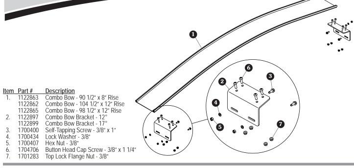
STEP 1: Place combo bow on top of trailer, across front. Determine mounting location according to depth of fabric cap packaging plus 10". Mark location on top rails.
