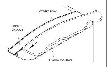
**NOTE:** Use one section of flat bar across straight portion on front of cap. Side and radius may be one section. Use as few sections as possible. Supply even tension over fabric cap for secure and clean fit.
