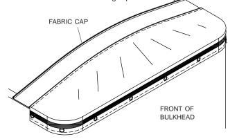
STEP 3: Hook tarp straps into D-rings on fabric cap.
