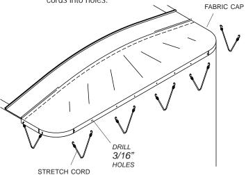
STEP 5: Locate rope anchors so stretch cords receive at least 10 pounds of pressure. Drill 1/4" holes and fasten rope anchors with screws ② and nuts ⑤. Hook stretch cords over rope anchors.
