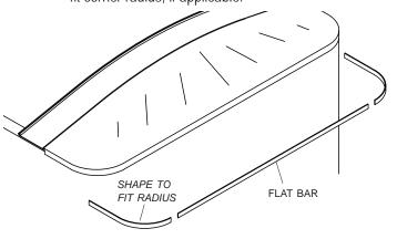
STEP 3: Work fabric cap over front of bulkhead. Align seam in fabric with weld along top of trailer.
