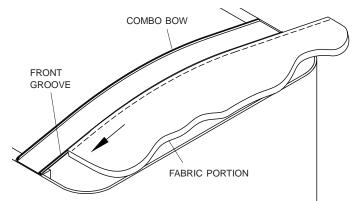
STEP 2: Work fabric cap over front of bulkhead. Align seam in fabric with weld along top of trailer.
