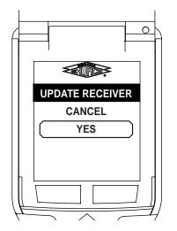
**STEP 2:** Wait for progress bars to update. Do not press any buttons on remote while progress bars are moving. When you see *Press Select*, press select button on your remote.
