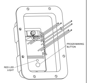
2. Check that receiver is connected to 12-volt power supply. Receiver must be connected to power to be programmed. If battery disconnect switch is installed, make sure it is turned on.
