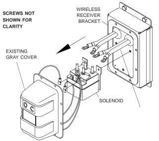
STEP 2: Install solenoid **②** onto wireless receiver bracket. Fasten with #10 x 1/2" cap screws. \_
