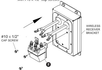
STEP 3: Connect wires from receiver bracket to solenoid and from gray solenoid cover to solenoid as shown below.
