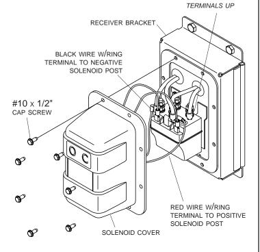
**NOTE:** Red and black wires with quick-disconnect terminals are taped and bent up inside grey cover above push button switch.
