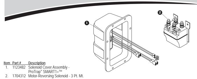
STEP 1: Disconnect power to ProTrap®. Remove existing gray cover and RF solenoid from ProTrap® intermediate bracket.
