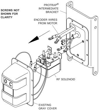
STEP 2: Install solenoid **②** onto ProTrap® intermediate bracket. Fasten with #10 x 1/2" cap screws.
