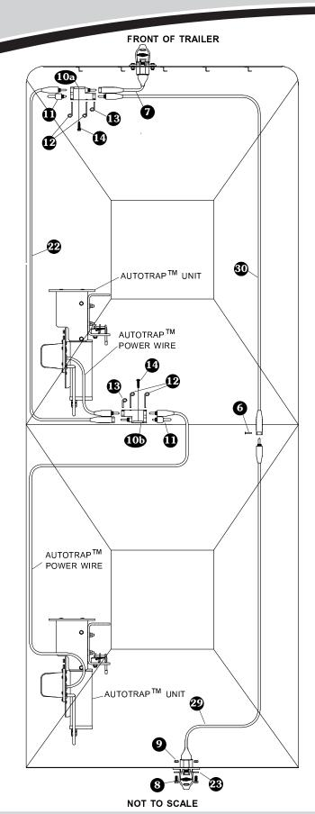
**NOTE**: Coat each connection with dielectric grease (P/N 1704378) to prevent corrosion.
