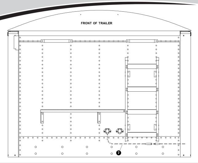
**NOTE:** Wire lengths are predetermined. Before installing SMARTwire™ components, review and confirm wire routing so that wires will reach components with ample room for connection.
