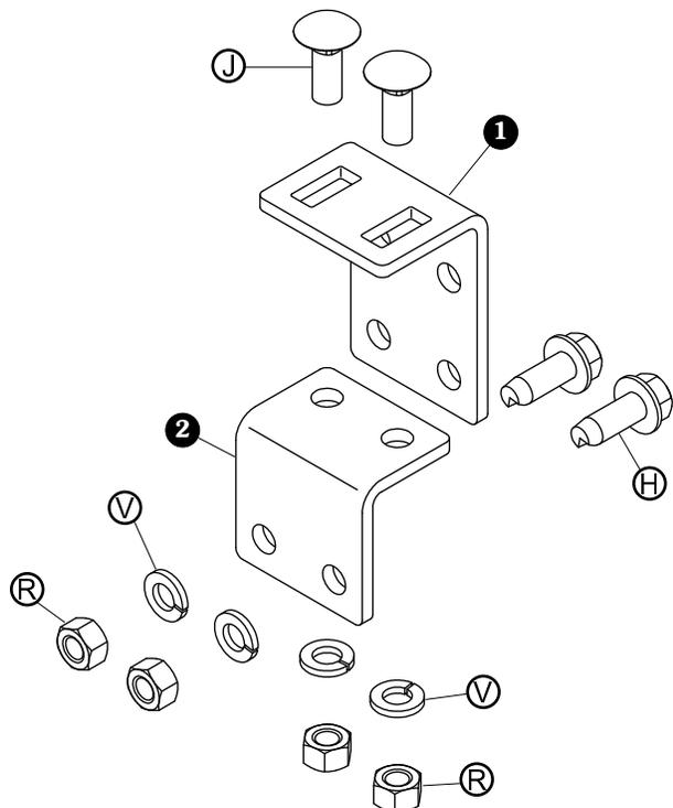
**NOTA:** Adjustable offset brackets create space between box and tarp stops/latchplates. Use where hinge gates interfere with standard tarp stop/latchplate installation.
