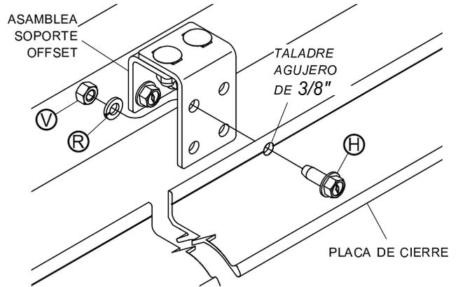
**NOTA:** Fasten latchplate to brackets through only one hole, in most cases. Where latchplate sections meet, fasten as shown.
