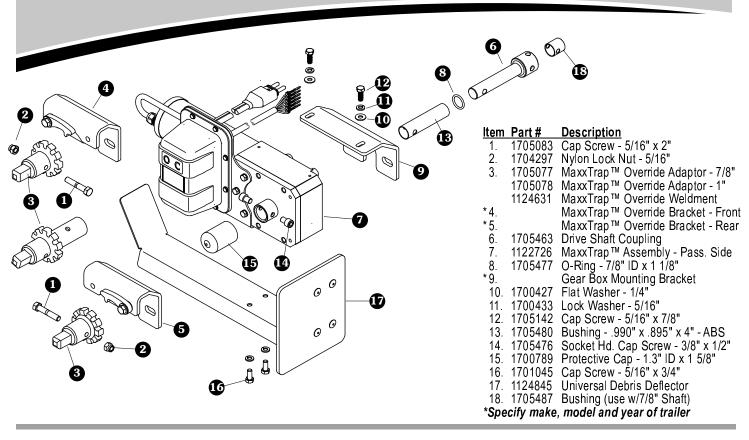
STEP 1: Install gear box mounting bracket **9** between bearing and hopper rail on passenger side (USA) of hopper. Install nuts and tighten just enough so bracket contacts hopper rail but can still move up and down.
