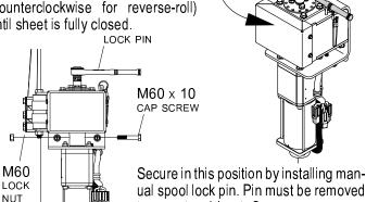
ual spool lock pin. Pin must be removed to open tarp/sheet. Or, you may secure pin in this position by reinstalling M10 x 60 cap screw and M10 lock nut. These must be removed to open tarp/sheet.
