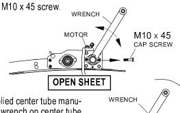
Using supplied center tube manual override wrench on center tube motor shaft, turn shaft clockwise (counterclockwise for reverseroll) until tarp/sheet is fully open.
