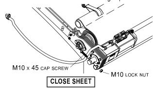
Use 17mm socket wrench on hex end of spool, turning spool clockwise (counterclockwise for reverse-roll) until sheet is fully closed.
