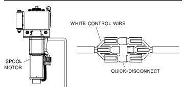
STEP 2: Disconnect power to receiver by unplugging SMARTwire™ connector.
