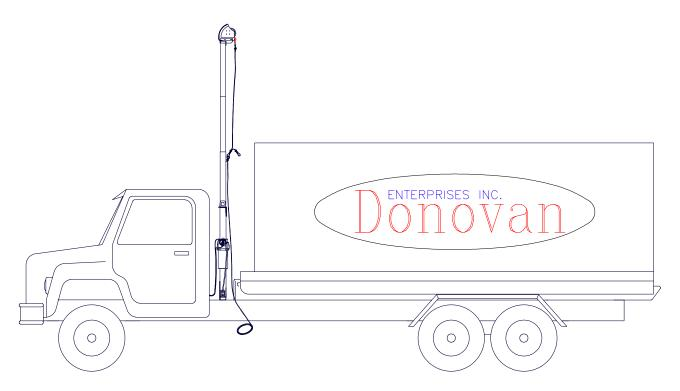
STEP 2: Use remote operating switch to raise HY-TOWER<sup>TM</sup> (SL) to its maximum height, while allowing rope to extend with tower (fig. 2).
