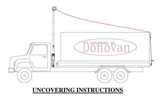
STEP 1: Use remote operating switch to raise HY-TOWER<sup>TM</sup> (SL) to its maximum height (fig. 6).
