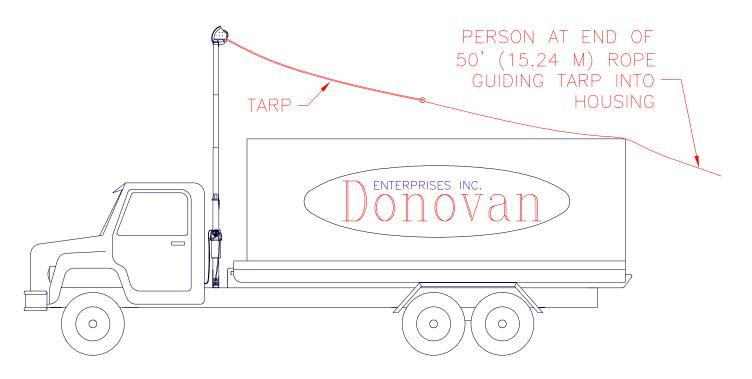
STEP 4: Use 50' (15.24 M) rope to guide tarp as it rolls up into housing (fig. 8).
