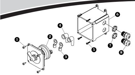
Item Part # Description 1704405 Self-Drilling Screw - Pan Hd. - #8 x 3/4" 1704283 Master Battery Disconnect Switch 1703244 Ring Terminal - 6 Ga. x 3/8" Stud Rubber Boot 1704330 1704338 Self-Tapping Screw - 1/4" x 1" Solar Master Disconnect Box 6. 1118556 Lock Nut - 1/2" 1704187 Dome Nut - 1/2" 1704152
