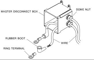
NOTE: Cut wires to length and strip only enough wire insulation to install ring terminals. Insert bare wire into ring terminals and crimp securely.
