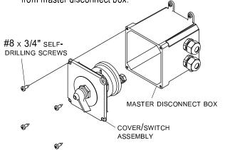
STEP 2: Run positive 6-ga. wire ends through dome nuts on master disconnect box. Run wire ends through rubber boots and crimp 16- to 14-ga. ring terminals to ends of wire.
