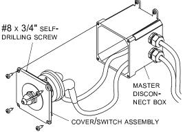
STEP 5: Locate master disconnect switch inside kingpin in easily accessible area. Fasten box to trailer with 1/4" x 1"
