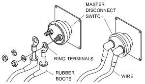
STEP 4: Reinstall cover/switch assembly to master disconnect box. Fasten with #8 x 3/4" self-drilling screws.
