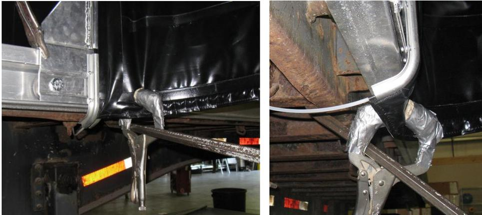
3. Insert the pry bar as shown and push down to bring the end of the tarp out past the end of the tarp holder
