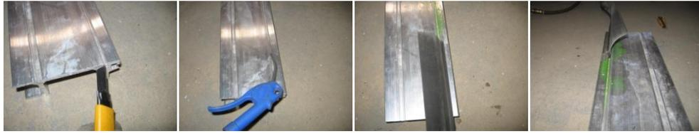
7. Insert the track rubber in the 48 ft. length of track allowing 6 to 8 inches of track rubber to extend beyond the front end.
