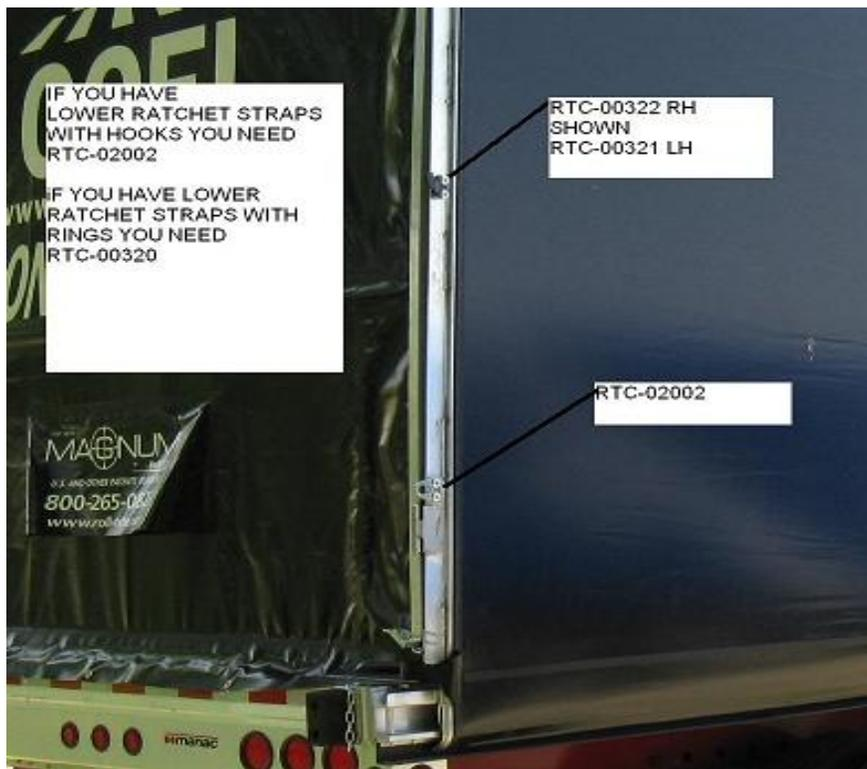
Note: Make sure that the over 90 bar will be able to pass freely when 4 washers per bolt are spaced behind the Hooks and Delta rings
