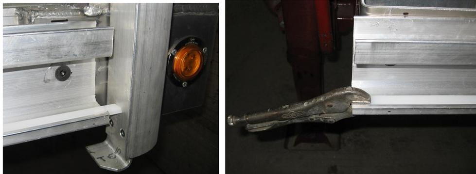
6. From underneath the track Drill a  $\varnothing$  9/32 hole up through the center of the nylon insert and insert a 1/4" flat head screw down through the hole and fasten with a nut so the screw head is flush with the insert.
