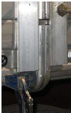
3. Slide the tarp holder in between the flat bar and up to the 1/2" mark made earlier to align the holder with the channel tube and clamp with the vice grip.
