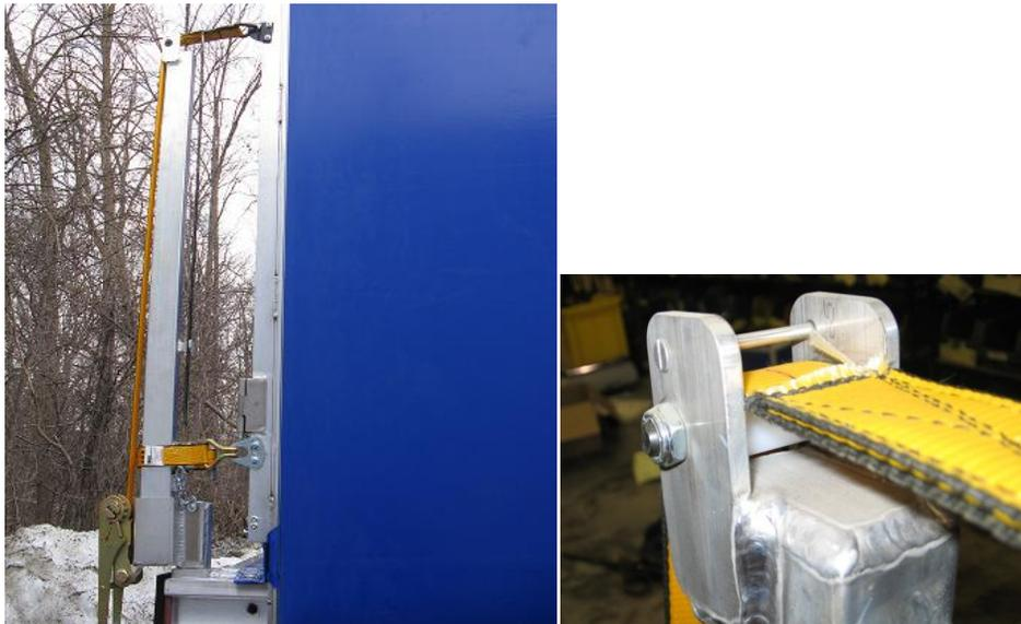
Note: the rod must be to the outside of the system away from the rear flap area
