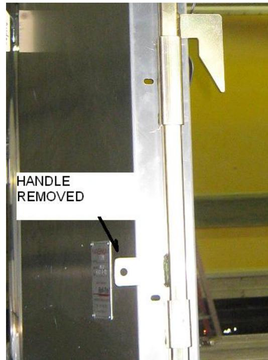
3. Slide the appropriate side frame (wing) onto the slide locks making sure to slide the bottom handle mount through the tarp seal on the inside of the side frame and out through the slot.
