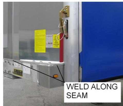
2. For aluminium trailers weld along the seam between the front of the trailer and the headboard mount plate. Grooving may be required to allow for better penetration of the weld.
