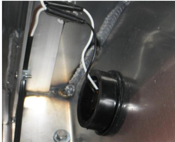
4. Feed the end of the harness through the hole in the corner of the headboard
