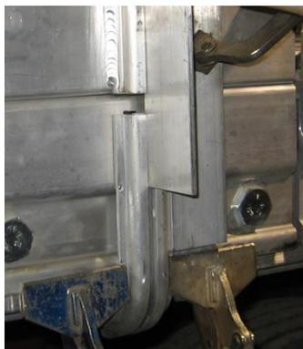
5. Remove one piece of flat bar and insert a piece of flat bar in the slots in the channel tube and tarp holder to insure correct alignment.
