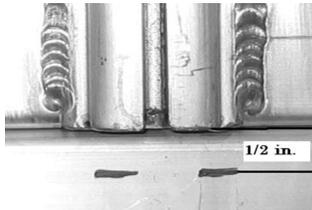
1. Measure down 1/2" from the bottom of the channel tube and place a mark on the foot below the channel tube. (mark all feet at the same time)
