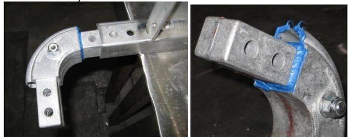
3. With a pair of corners sealed, install in the tubes and fasten with the hardware provided.
