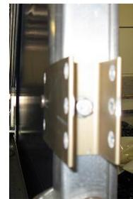
Note: Turn the clevis pins so that the holes face the front and the back of the trailer
