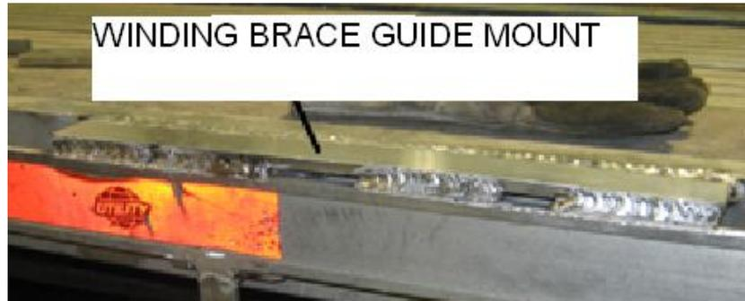
6. Install the guide rail mount **30"** for **72 or 100H** or **40"** for **Drop Deck** from the rear of the Base Plate in the same manner as the base plate.
